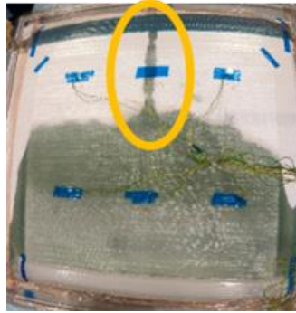
Figure 2: Flat infusion with a nominal gap between balsa panels, highlighting the advanced flow front.
